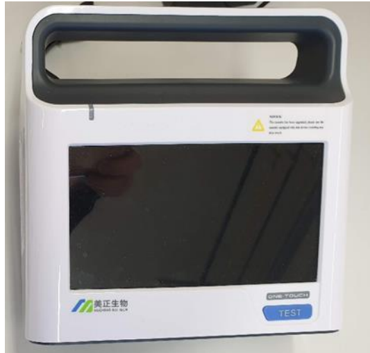
Fig. 2. BMZ6000 Portable Strip Reader for instrumental reading of the color formation on the AnticFast® Beta-lactams & Tetracyclines Combo Test Kit.
